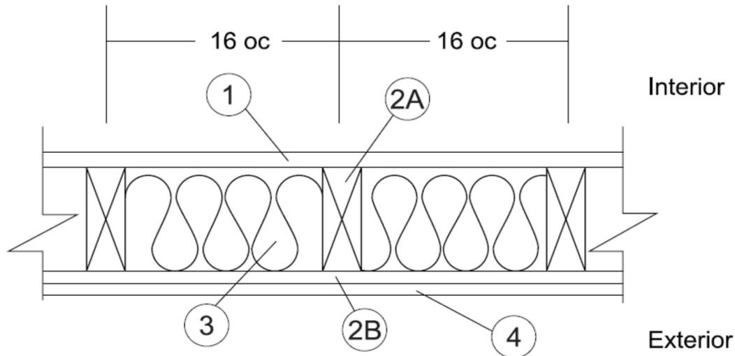
1. **GYP SUM BOARD (Interior):** One-layer Type X complying with ASTM C1396, min.  $\frac{5}{8}$  in. thick, 4 feet wide applied vertically, fastened to framing. Joints covered with paper tape and joint compound. Fasteners covered with joint compound. Min. #6 x  $1\frac{5}{8}$  in. long Type S or W screws, spaced max. 6 in. on center o.c.
