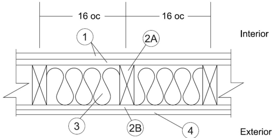
**1. GYPSUM BOARD [Interior]:** Two layers Type C USG Firecode® C Core complying with ASTM C1396, min. 5/8 in. thick, 4 feet wide applied vertically, fastened to framing. Face layer joints staggered with base layer and covered with paper tape and joint compound.
