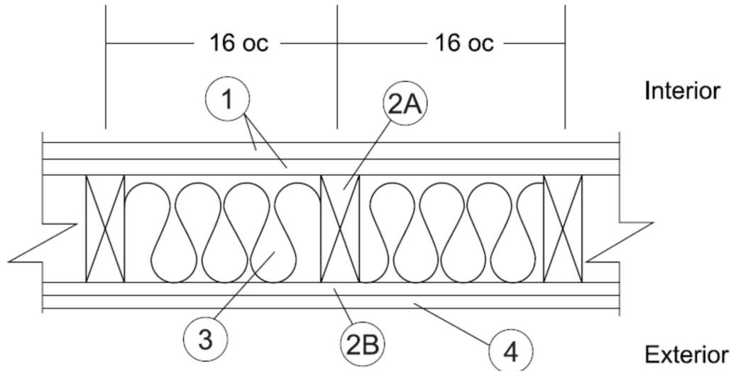
**1. GYPSUM BOARD (Interior):** Two-layers USG Firecode® C Core, complying with ASTM C1396, or equivalent, min.  $\frac{5}{8}$  in. thick, 4 feet wide applied vertically, fastened to framing. Face layer joints staggered with base layer and covered with paper tape and joint compound.
